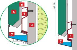
Figure 1. Structure of plant cassettes on the outside of an existing wall. (Source: Optigreen)
